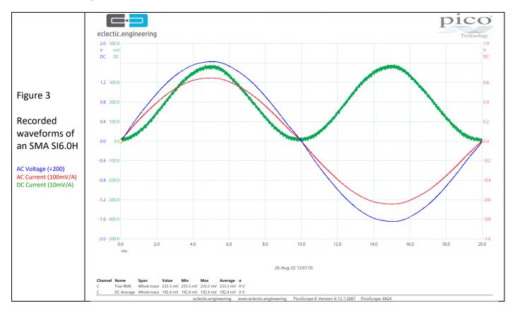
Here the Average DC current as calculated by the Picoscope above is 192.4mV (÷10mV\*1A) which is 19.2A and the RMS value is 233.3mV (÷10mV\*1A)
