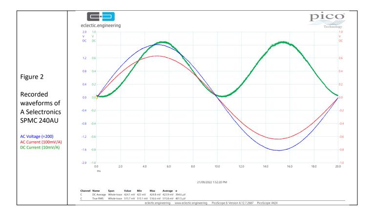
The Average DC current as calculated by the Picoscope above is 423.9mV (÷10mV\*1A) which is 42.4A and the RMS value is 515.8mV (÷10mV\*1A)
