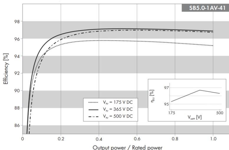
Figure 7.10: Example of an inverter efficiency curve (SMA Sunny Boy 5.0-1AV-41).
