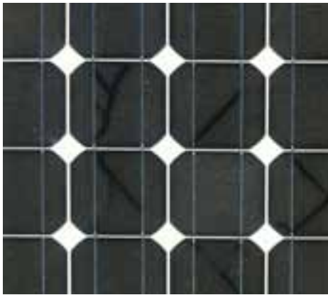
Figure 1: Example of module discolouration or 'snail trails' on modules.
