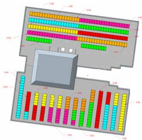
**Figure 6. String layout, designating modules to selected inverter and string.**
