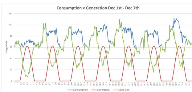
**Figure 8. Data from an interval analysis of the comparison of consumption and generation data collected using a power analyser or interval meter.**
