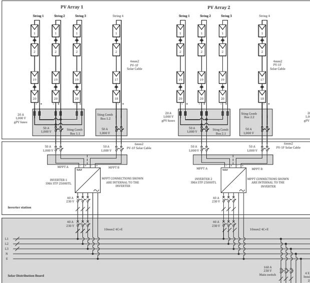
**Figure 3. Single Line Diagram (SLD) depicts the electrical connections between the PV array, inverter, electrical protection equipment and MPPTs.**
