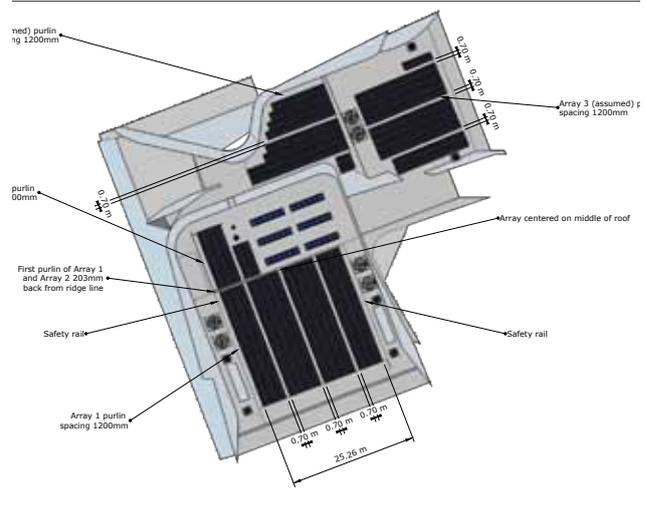
Figure 1. 3D view of object or structure (i.e. the PV Array and related structures) as seen from above.
