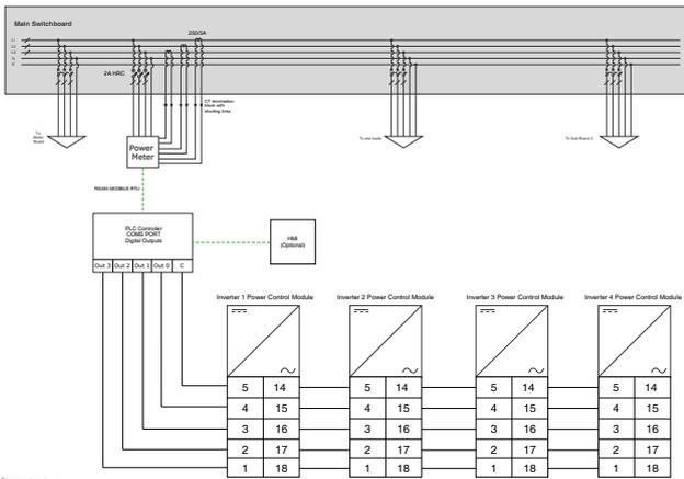
**Figure 4. SLD of the electrical schematic of a custom zero export device.**
