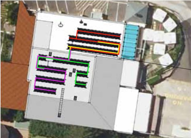
**Figure 7. Module and wiring layout with directions for roof entry point.**
