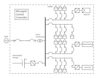
supercapacitors or flywheels. Electric vehicle batteries can also serve as this energy storage. In island mode, microgrids often have no inertia or spinning reserves; that is, they are unable to provide for the instantaneous loss of renewable generation. Energy storage can make up for this lack of inertia by providing the necessary energy until another source can provide the required energy.
