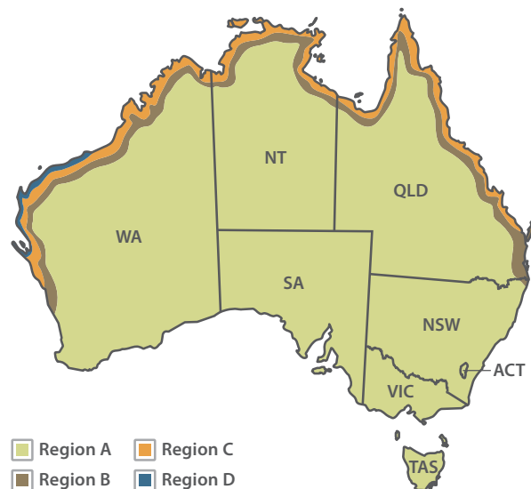
Figure 1: Map of Australia showing the four different wind regions. A more detailed version of this map showing regional centres can be found in AS/NZS1170.2: (Section 3.2)
