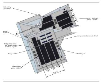
Figure 1. 3D view of object or structure (i.e. the PV Array and related structures) as seen from above.
