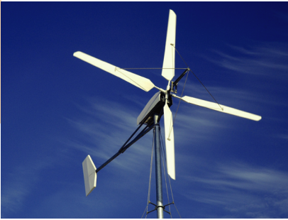
Figure 5.10: Pawicon 2.5kW Upwind Turbine. (Source: Paul Gipe, WindEnergy)
