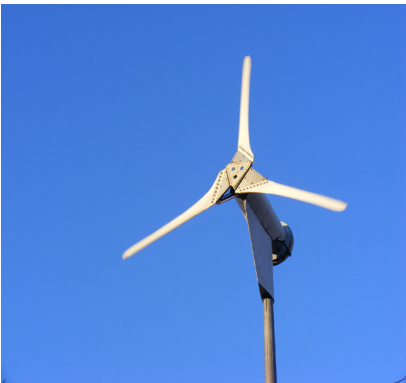
Figure 5.11: Proven 6 kW Downwind Turbine (Source: Tobi Kellner [CC BY-SA 3.0], via Wikimedia Commons).
